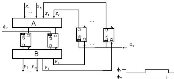
$$t_{CWH}(\phi_1) \geq t_{CWL}(\phi_2) + t_{skew}$$
